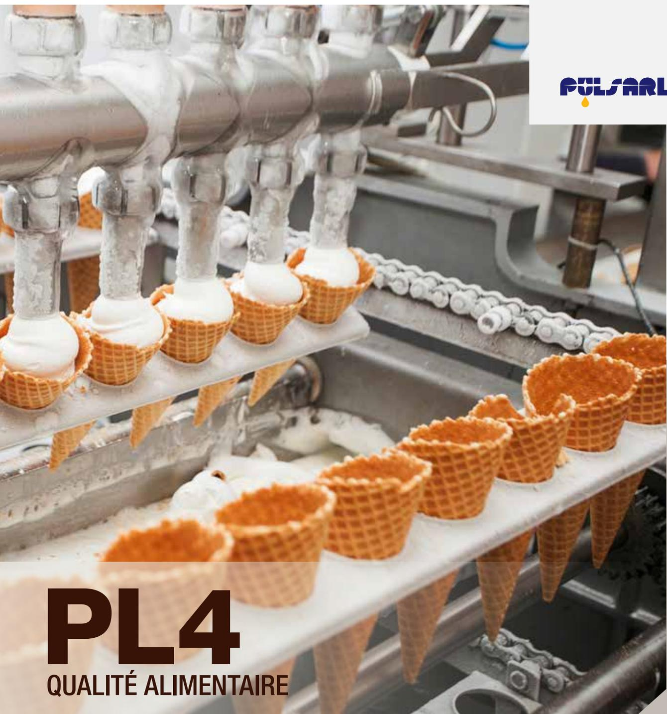
A detailed photograph of an industrial ice cream production line. Multiple metal dispensing nozzles are shown in the foreground, each dispensing a dollop of white ice cream into a golden-brown wafer cone. The cones are arranged on a white conveyor belt. In the background, more machinery and a chain of rollers are visible, creating a sense of a busy, automated factory environment.
