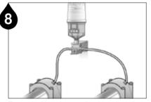
For typical bearing applications, install the divider block to the equipment using either copper or nylon tubes.
