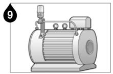
For motor bearing applications, install the mounting bracket at a proper location using the 2 point remote installation kit and then connect the lube-lines to both bearings.
