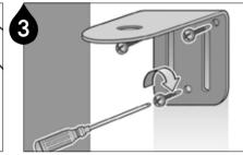
Install the mounting bracket (B002) at a proper location using screws (B051).
