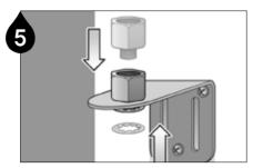
Install the adaptor (A002) on the fixed mounting bracket with the washer (B058) on the bottom.
